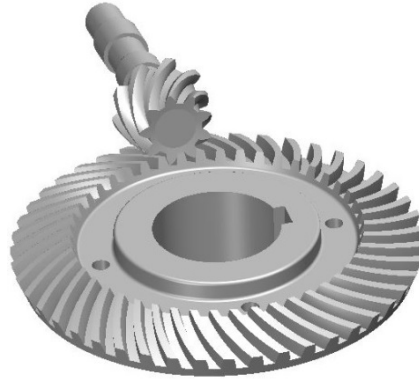
Figure 7. 3D model of the spiral bevel gear model created in SINOvation
